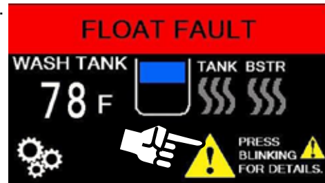
Fig. 99 - Fault screen with blinking icon
